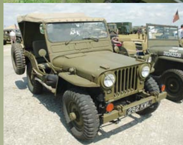
Bottom group: the French-built M201 Hotchkiss Jeep is the most widely available post-war Jeep, and while some models were built to incorporate a recoilless gun (below left), and some were fitted with roll over bars (bottom left), most were virtually identical to the original wartime Jeep.
