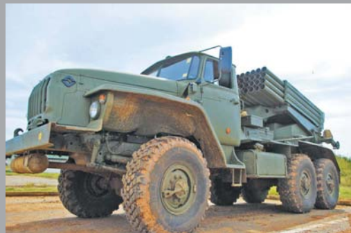
Above: the BM-21 122mm Grad multiple tube rocket launcher is based on the Ural truck, which provides a commonality of parts with the cargo trucks.
