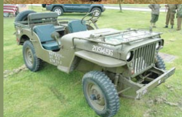
Left: the Willys CJ-2A was a post-war Jeep and while it looked very similar to the original wartime Jeep, it corrected many of the original Jeeps faults. A drop down tailgate, and drain holes in the footwells were just two of the modifications.
