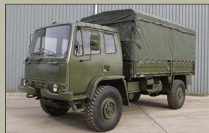
Leyland Daf 45 / 150 4x4 Cargo, Fitted Power Steering, Hi/Lo diff lock, 3 seats, air brakes, rear Nato style hitch, spare wheel, etc, Good condition. Guide price from £5,750 Also Available Leyland Daf 45 / 150 4x4 Flatbed, price from £4,750 (100 Available)
