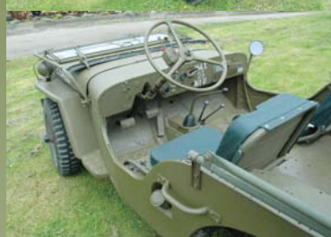
Left: in this view of a CJ-2A we can see the side fuel filler, which is an easy way to distinguish it from the wartime Jeep.
