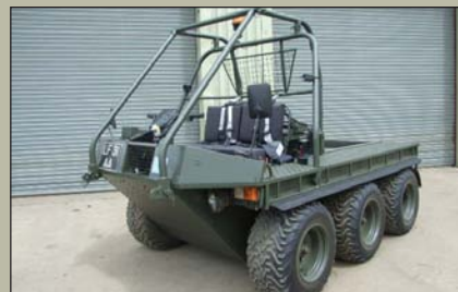
Supacat 6x6 ATMP fitted VW 1.9 turbo diesel, auto gearbox, 1 ton load capacity, fitted roll over frame, some fitted winch. Guide price from £9,500 (5 Available)
