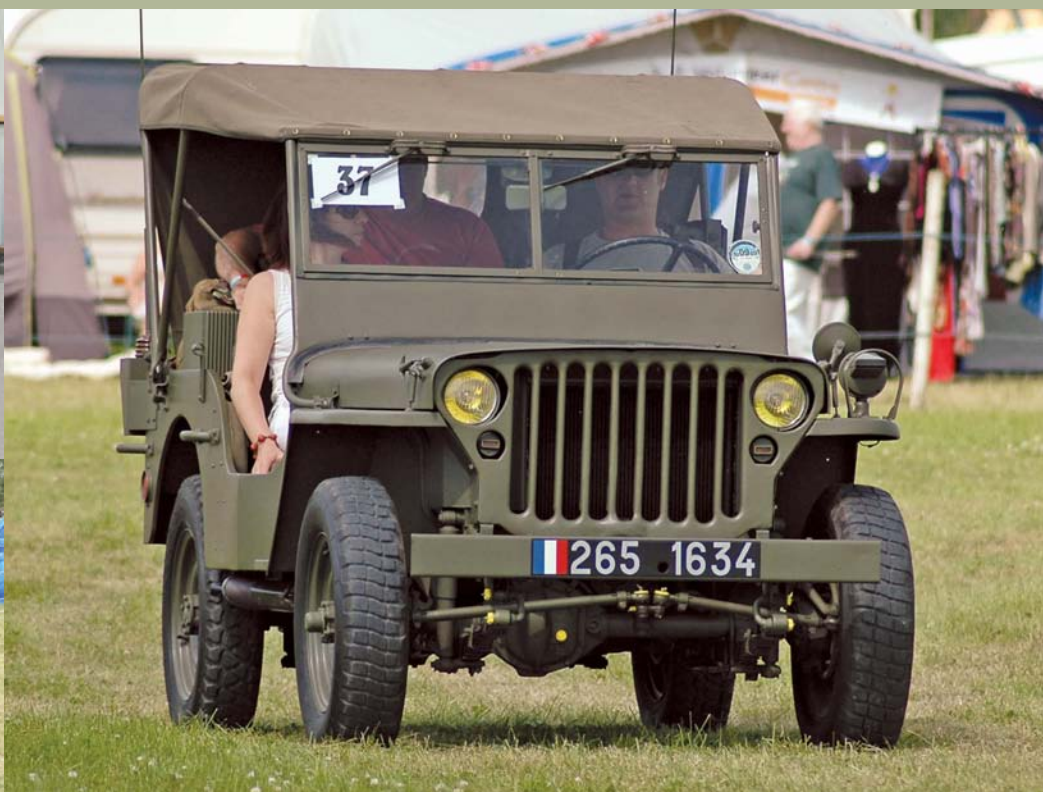
Bottom group: the French-built M201 Hotchkiss Jeep is the most widely available post-war Jeep, and while some models were built to incorporate a recoilless gun (below left), and some were fitted with roll over bars (bottom left), most were virtually identical to the original wartime Jeep.
